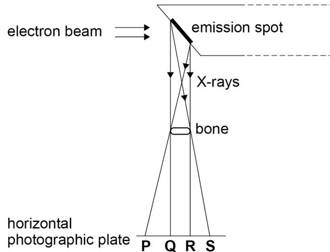
**Figure 3** shows how a total shadow is produced in the region **QR** where no X-rays from any part of the emission spot can reach the photographic plate. Partial shadows are formed in regions **PQ** and **RS** where X-rays from only part of the emission spot can reach the plate.
