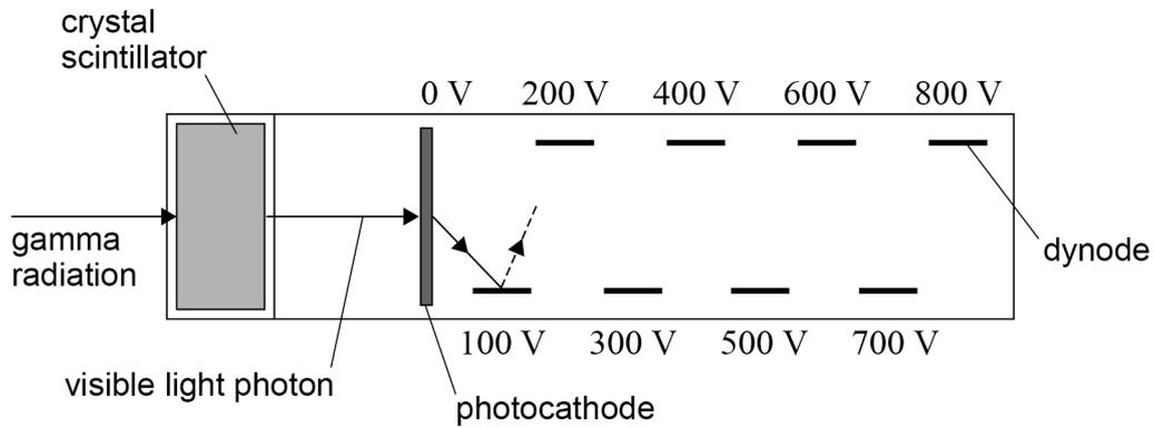
At the crystal scintillator, each photon of gamma radiation leads to the emission of one visible light photon.
